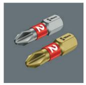
BTH- (extra-hard) and BTZ- (tough) bits have an additional tempered BiTorsion zone, which reduces the hardness of the shaft by about 20 % in comparison to the drive tip. This means that the peak loads that cause bit breakage and premature wear are absorbed in this zone - something which enhances the service life of the bits.
